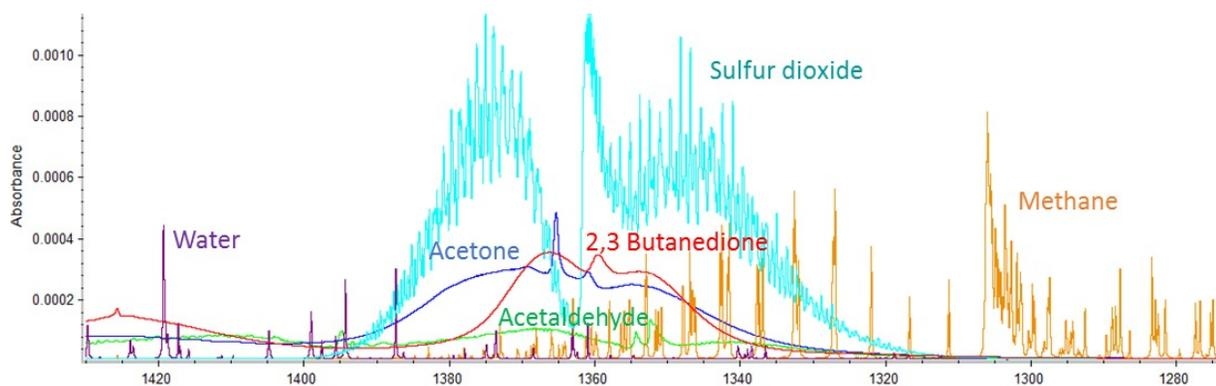
Figure 4. Spectral library of molecular species of interest in the tuning range of the ECQCL used in this study.
