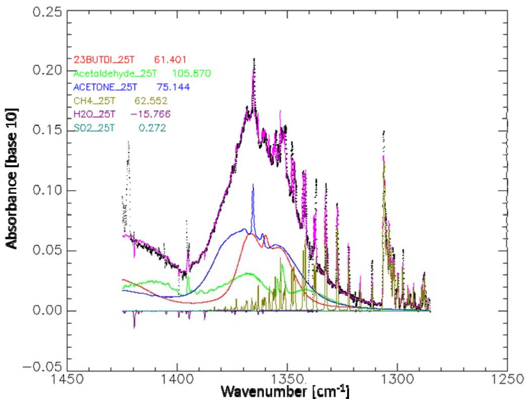
Figure 6. Example library fit to the sample spectral data that is shown above in Figure 5. Measured absorption is shown as black points and the composite quantitative fit is shown with the overlaid magenta line. Also shown is a representation of the contributing parts to this fit for the different library species with the legend listing the calculated concentration in ppm.
