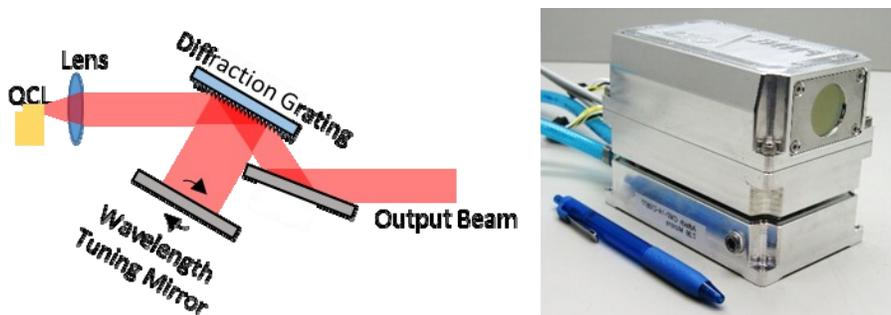
Figure 3. Diagram of PNNL ECQCL Littmann-Metcalf cavity, alongside a picture of an ECQCL produced jointly by OptoKnowledge and PNNL.
