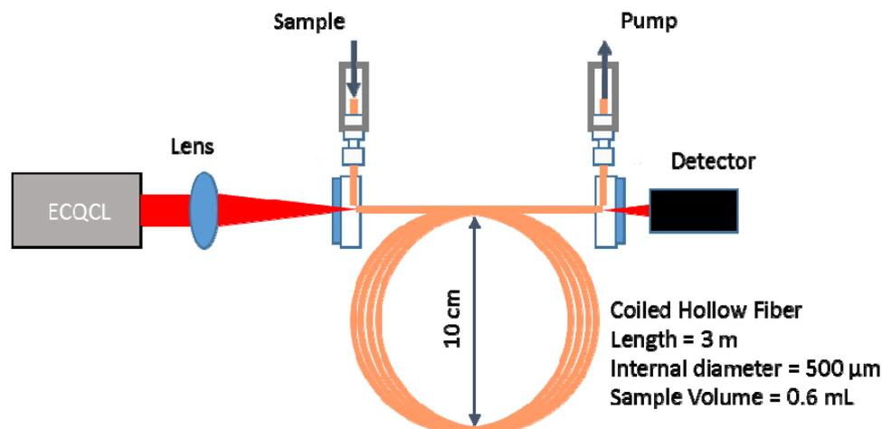
Figure 1. Diagram of versatile CAS+ECQCL system for the analysis of multiple gasses with an ultra-small sample volume.
