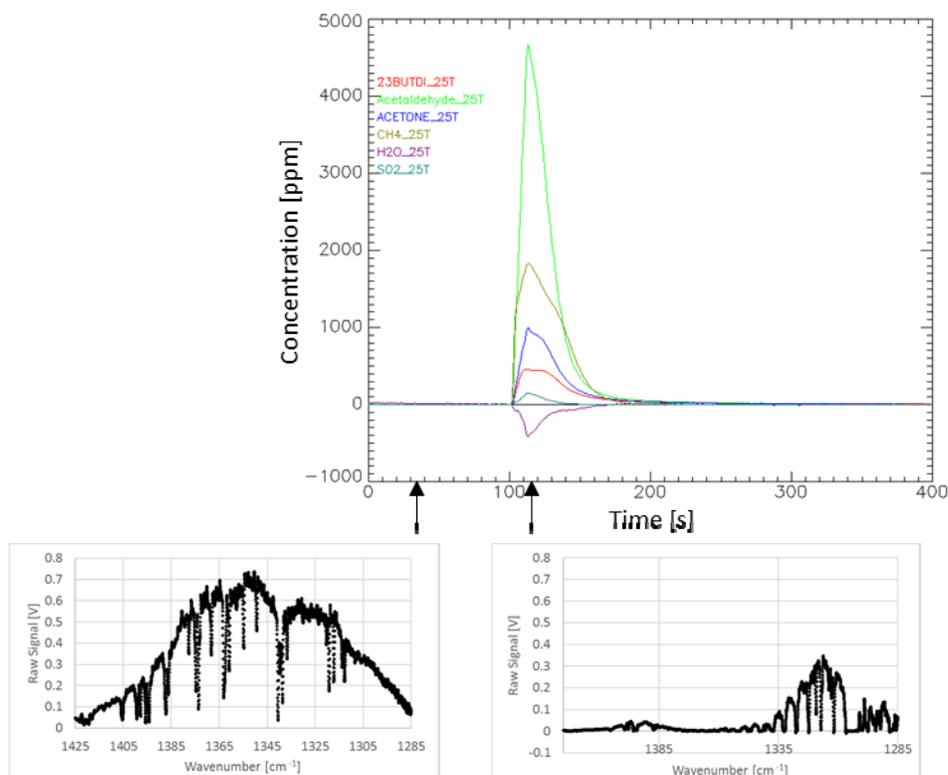
Figure 7. Measured concentration versus time demonstrating the high dynamic range and ability to determine concentration in the presence of strong absorption. Inserts show transmission spectra before and at peak concentration.
