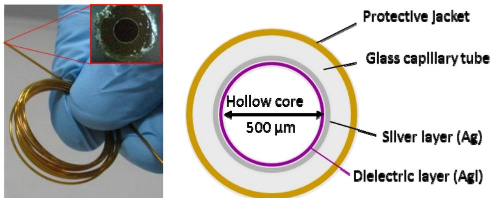
Figure 2. Picture of tightly coiled hollow fiber alongside cross-sectional diagram.
