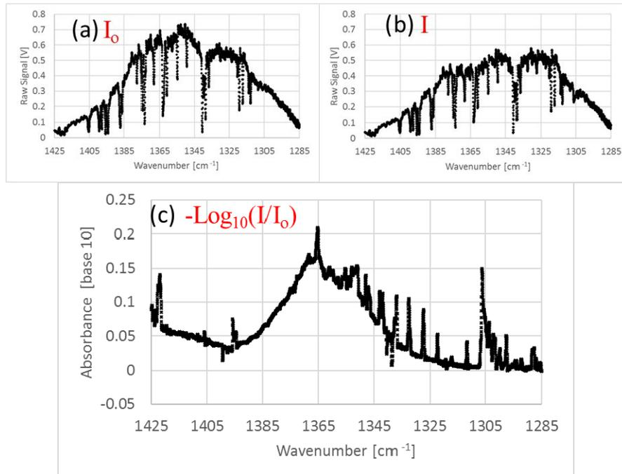
Figure 5. Sample data: (a) “Background” transmission spectrum ( $I_0$ ) taken with room air circulating through cell, the strong absorption features are due to water vapor, (b) measurement spectrum ( $I$ ) taken after a sample was introduced into the fiber gas cell, (c) Absorbance spectrum calculated as  $-\text{Log}_{10}(I/I_0)$ .
